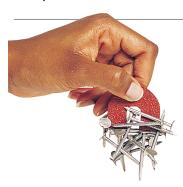
A magnet can be used to separate a mixture of the elements iron and aluminum. Iron is attracted to the magnet, but aluminum is not.
