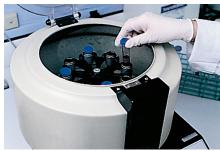
Blood is separated into its parts by a machine called a **centrifuge** (SEN truh FYOOJ). In the test tube of blood at left, a layer of plasma rests atop a layer of red blood cells. A centrifuge separates mixtures by the densities of the components.
