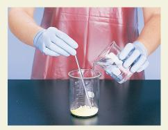
**Dissolving** In the first step, water is added, and the mixture is stirred. Salt dissolves in water. Sulfur does not.
