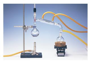
**Distillation** (DIS tuh LAY shuhn) is a process that separates a mixture based on the boiling points of the mixture's components. Pure water (flask on the right) is being distilled from salt water (flask on the left). Also, distillation is used to separate crude oil into components, such as gasoline.
