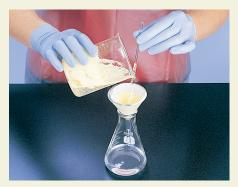
2 Filtering In the second step, the mixture is poured through a filter. The filter traps the solid sulfur.
